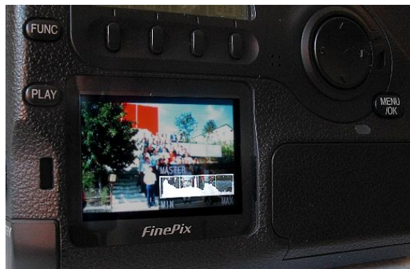
Fig. 1: Digital camera back display showing a histogram overlay
