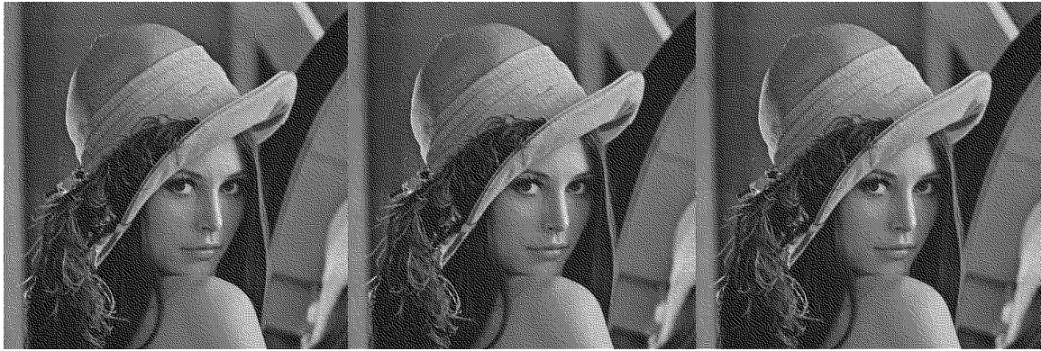
Fig. 11: Floyd-Steinberg algorithm applied on image “Lena.bmp” (a) threshold 125 (b) threshold 80 (c) threshold 60
