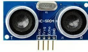
Figure 4. HC-SR04 ultrasonic sensor 4
