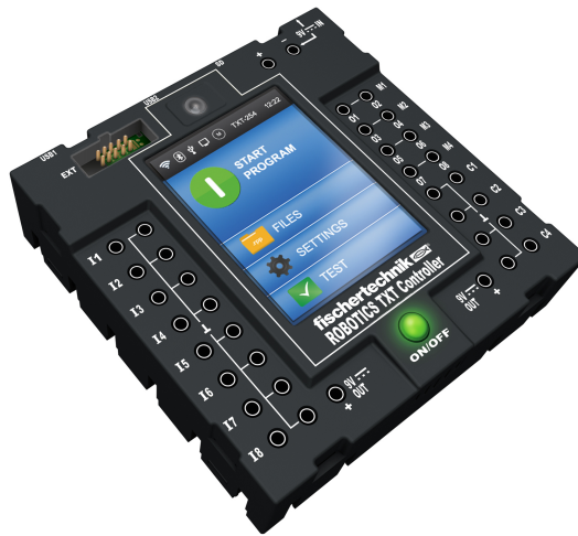
Fig. 1: Fischertechnik TXT-Controller: Dual processor ARM Cortex A8 + Cortex M3, 8 universal inputs (digital/analog) I1 ... I8, 4 fast counting inputs, 4 motor outputs, BT 2.1 EDR+ 4.0, WLAN 802.11, Infrared receiver diode, USB 2.0 Client, colour touch display [5].
