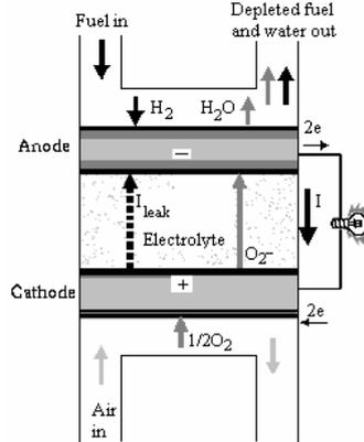
Fig. 2. Principle of a solid oxide fuel cell
