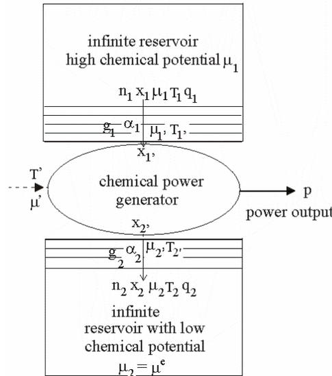
Fig. 1. A scheme of an engine controlled by a suitable choice of Carnot variables  $T'$  and  $\mu'$ .
