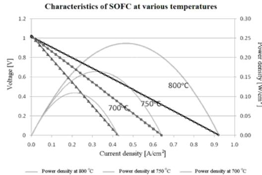
Fig.3. Voltage-current density and power density characteristics of the SOFC for various temperatures. Continuous lines represent the Aspen Plus<sup>TM</sup> calculations testing the model consistency with the experiments. These lines were obtained in Wierzbicki's MsD thesis supervised by S. Sieniutycz and J. Jewulski [14]. Points refer to experiments of Wierzbicki and Jewulski in Warsaw Institute of Energetics ([14] and ref [18] therein).
