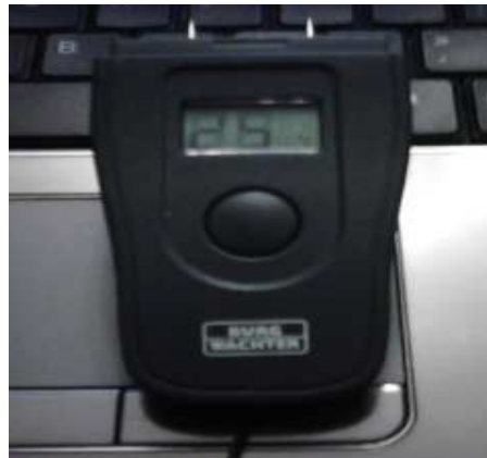
Figure 1. Burg Wächter device[7] for temperature direct measurement
