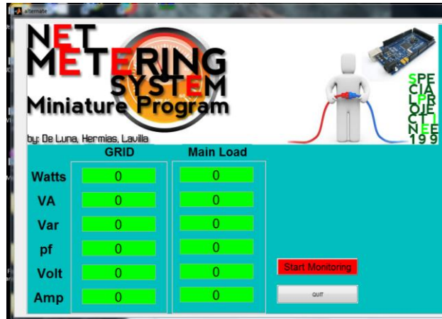
Fig. 4. GUI of the Matlab Monitoring Program
